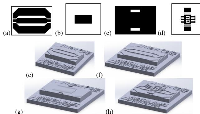
Fig. 4. (a) to (d) Photomask layouts generated in SolidWorks, (e) to (h) 3D models for each layer required for the fabrication of the MEMS switch.
