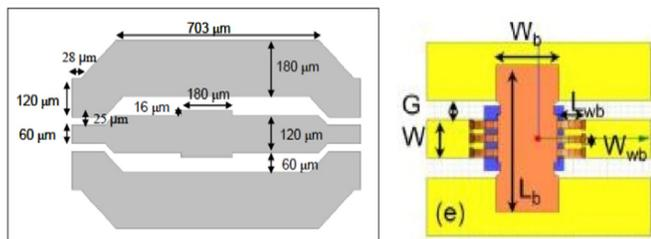
Fig. 3. Original dimension layouts of the MEMS switch bridge, signal and ground lines [10].
