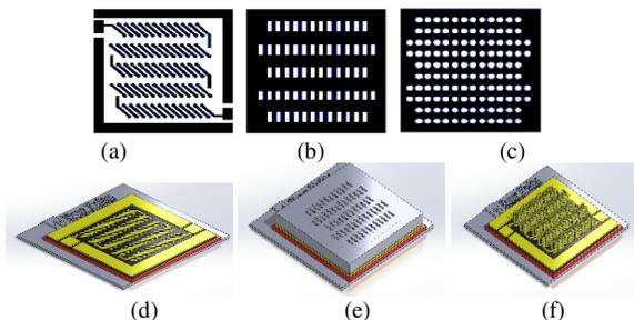
Fig. 6. (a) to (c) Photomask layouts generated in SolidWorks, (d) to (f) 3D models for each layer required for the fabrication of the MEMS inductor.
