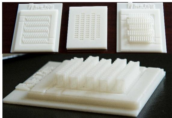
Fig. 7. 3D print of the scaled-up MEMS inductor, layer-by-layer and fully integrated and released.
