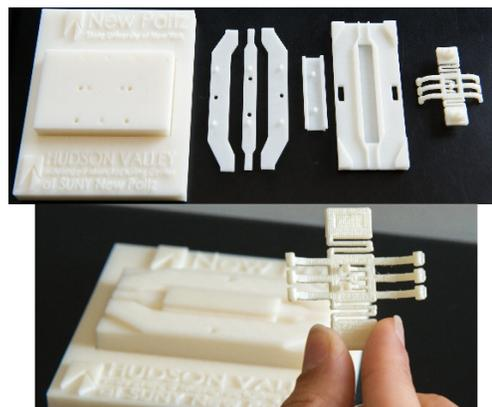
Fig. 5. 3D print of the scaled-up MEMS switch with an overall footprint of 5cm by 5cm.
