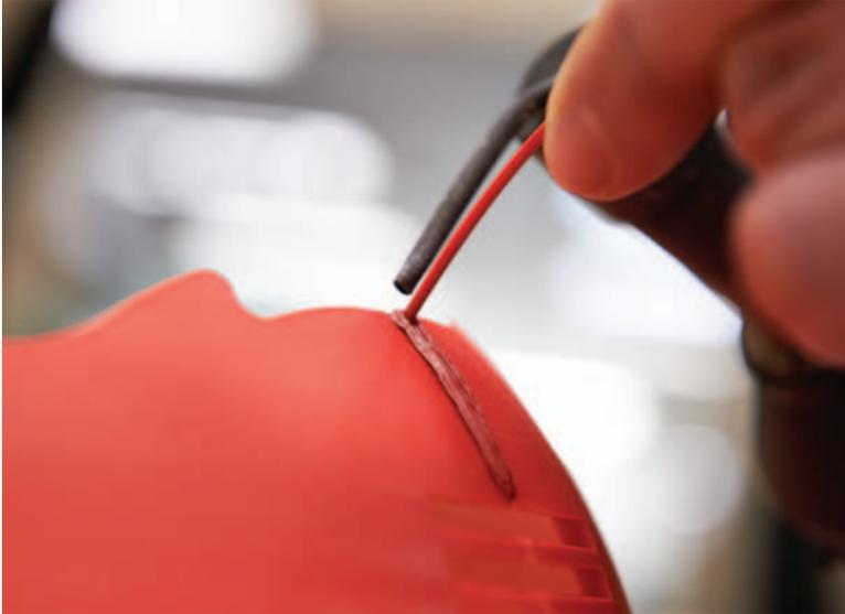
HOT AIR WELDING A SEAM
