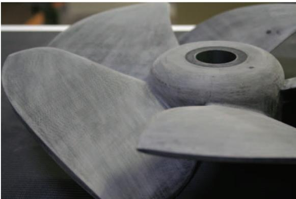
FAN PROTOTYPE PRODUCED WITH FDM
