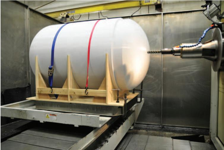
LOCKHEED MARTIN FUEL TANK SIMULATION BUILT IN TEN SECTIONS, HOT AIR WELDED TOGETHER AND MACHINED TO THE DESIGN'S CRITICAL DIMENSIONS
